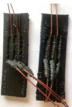
Peel Test for evaluating Adhesion
